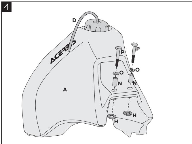
**Fix the Acerbis fuel tank (A) to the frame using the screws (P), the washers (O), the spacers (N) and the gaskets (H).** Screw the cap with the rubber tube (D). Remount the seat and the original side panels.
