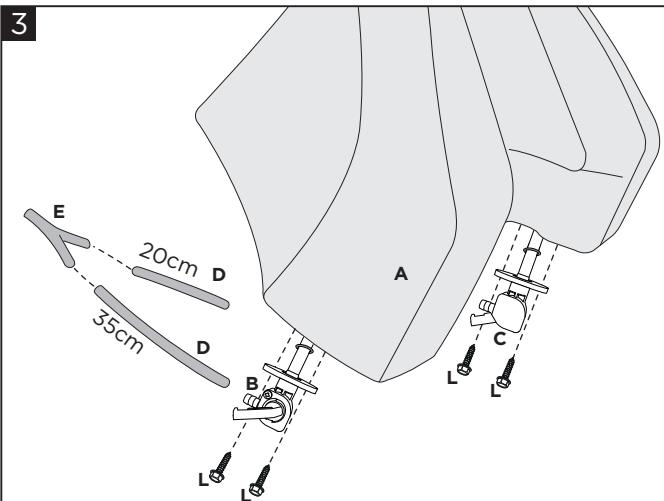
**Insert the taps (B) and (C) into the Acerbis fuel tank (A) using the screws (L).** Rest the tank on the frame and connect the taps to carburetor through the fitting (E) and the rubber tube (D), cut in the measurements indicated in the figure.
