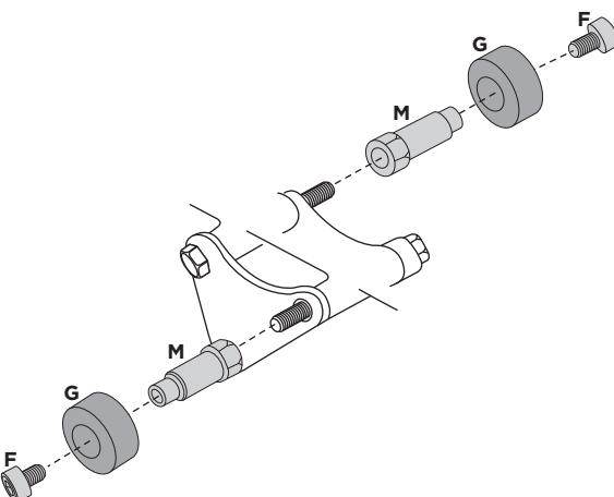
**Take off the original sell locking nuts and tighten the bearings (M), with the grommets (G) and the screws (D).**
