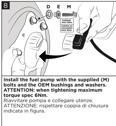
**Install the fuel pump with the supplied (M) bolts and the OEM bushings and washers.**
