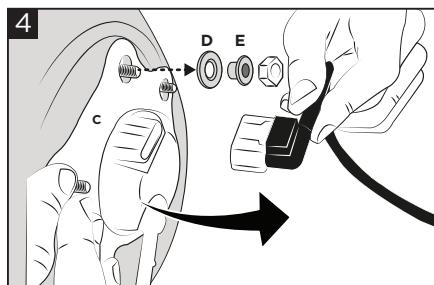
**Make sure the fuel has been removed from the tank, then disconnect the power cable from the fuel pump hardware (D) and (E).**
