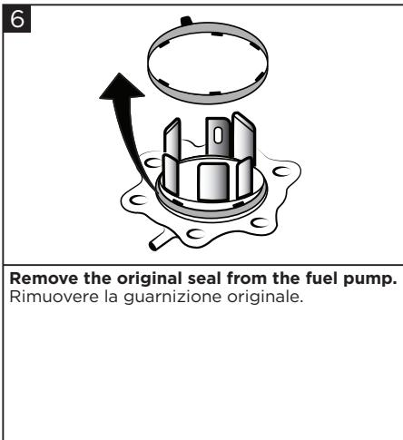
**Remove the original seal from the fuel pump.**
