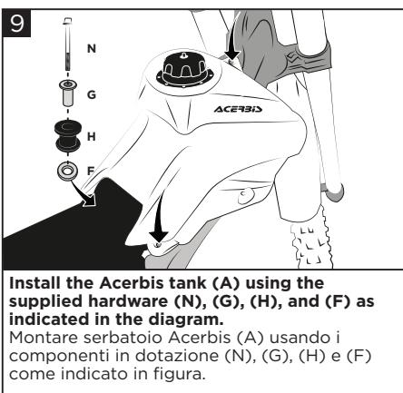
**Install the Acerbis tank (A) using the supplied hardware (N), (G), (H), and (F) as indicated in the diagram.**
