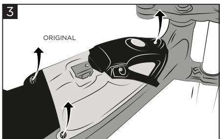
**Unscrew the tank screws and remove the OEM fuel tank.**
