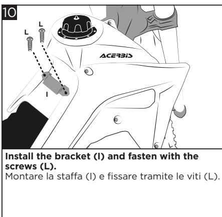
**Install the bracket (I) and fasten with the screws (L).**
