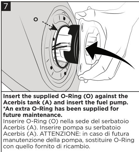
**Insert the supplied O-Ring (O) against the Acerbis tank (A) and insert the fuel pump.**
