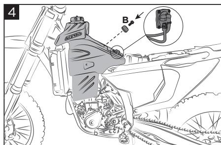
**Place the Acerbis tank (A) on the bike, secure it with the screw + rubber (B) and connect the pump to the connectors.**
