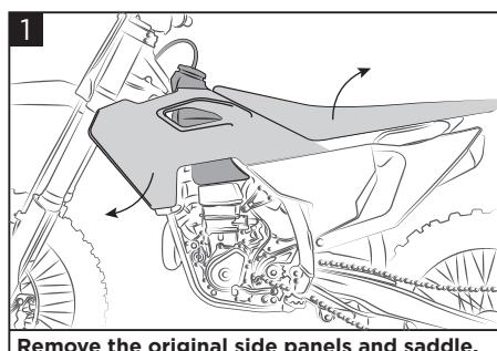
**Remove the original side panels and saddle.**
