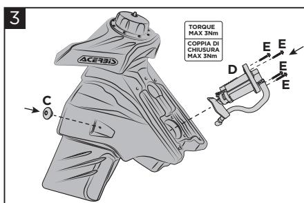
**Refit the screws (C) and the pump (D) on the Acerbis tank (A) using the screws (E).**
