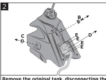
**Remove the original tank, disconnecting the pump connectors and unscrewing the screw and the rubber (B). Completely empty the tank from the petrol and remove the pump (D) through screws (E). Finally remove the screws (C).**
